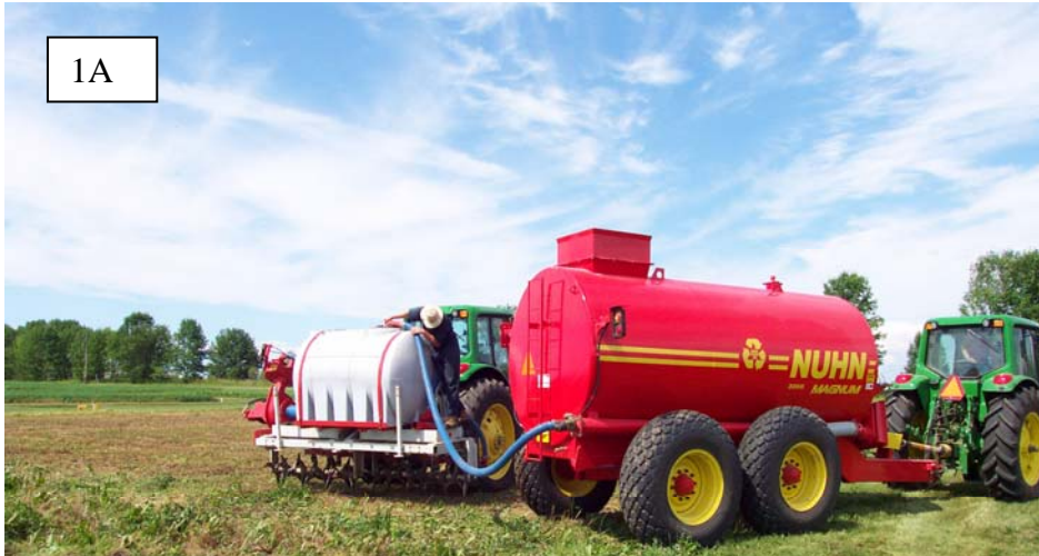
Figure 1. Photos of custom-built aeration-liquid manure application unit. 1A. Refill of the manure reservoir tank. 1B. View from side showing the agitator, metering unit and aerator. 1C, 1D. View of plots immediately following the aeration + manure treatment.
