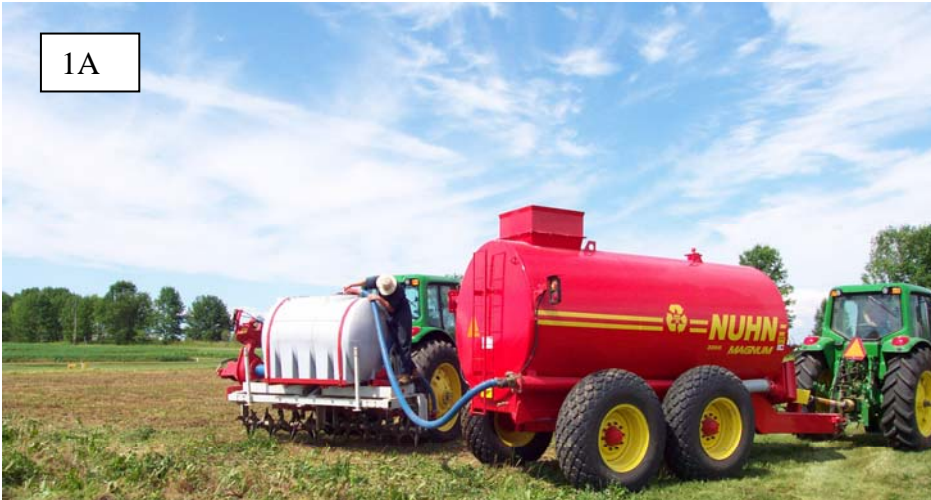
Figure 1. Photos of custom-built aeration-liquid manure application unit. 1A. Refill of the manure reservoir tank. 1B. View from side showing the agitator, metering unit and aerator. 1C, 1D. View of plots immediately following the aeration + manure treatment.
